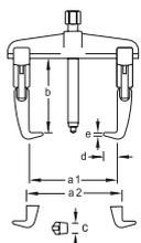
> Consisting of 5 pullers in different sizes with standard or quick-release pulling hook or all-steel hook with hook brake
