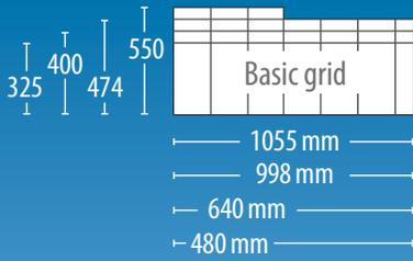
The drawer sizes and module variants are shown using a common basic grid.
