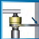
The L-form is also ideal for those points above the screwtightening level. However, the resulting tilting moment causes the max. permitted torque to drop by 20 %.
