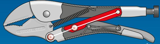
Self-clamping effect – can only be cancelled by operating the releasing lever!
