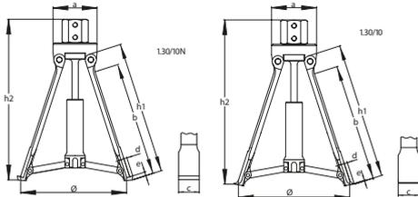
> Suitable for removing large ball bearings and bearing outer races
