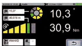
Virtual progress bar for torque and angle
