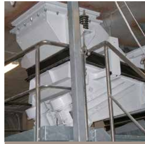
Regelbare Unwuchtrinne Unbalanced motor feeder with stepless capacity adjustment
