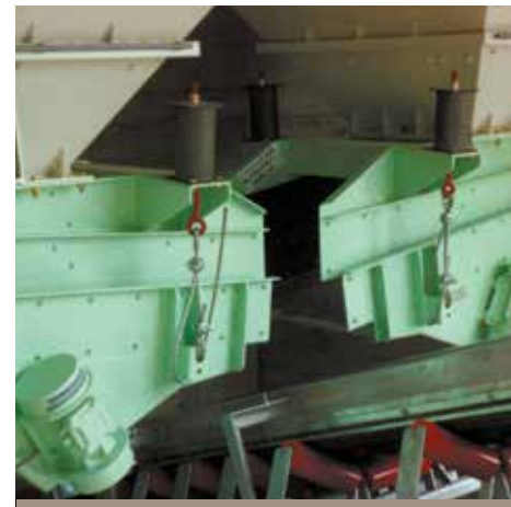
Unwuchtrinnen in offener Ausführung Unbalanced motor feeders in open design
